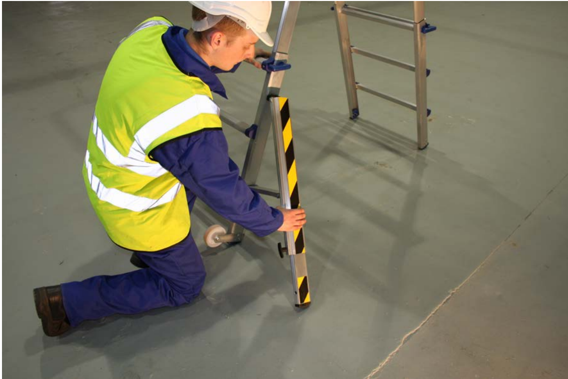
...and push down on the lower arm, until the leg extends, locks...
