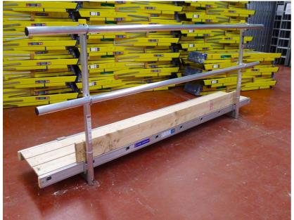
No tools required to fit, the Handrail Posts simply clamp to the underside of stagings. Inbuilt holders for toe-boards are included.
